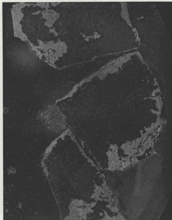
Fig. 11. Cross section of 50% \text{Al}_2\text{O}_3 and 50% \text{ZrSiO}_4 thermite pellet after heating to 2500°F. for 3 hours.
