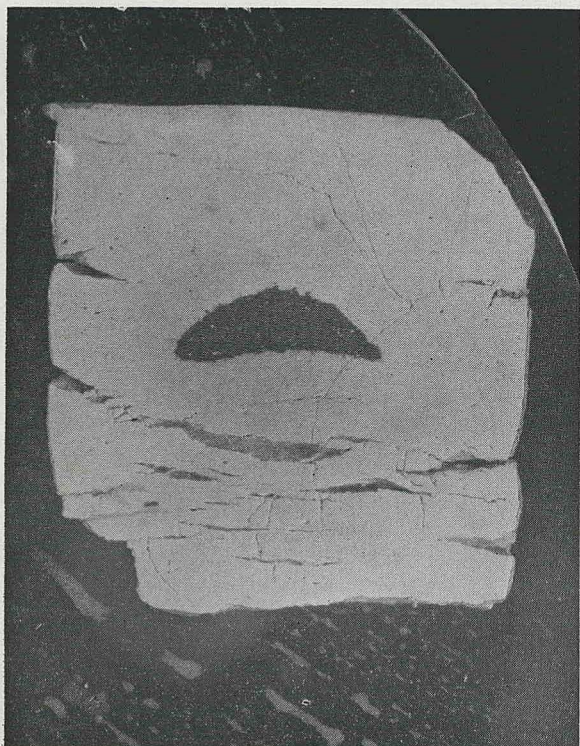
Fig. 7. Cross section of 50% \text{Al}_2\text{O}_3 and 50% \text{TiO}_2 thermite pellet after heating to 2500°F. for 3 hours.
